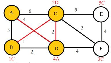
$\begin{array}{c|cccc} & \text{Vertex:} & F & E \\ \text{Queue:} & \text{cost:} & 3 & 5 \\ \text{prev:} & C & C \end{array}$
